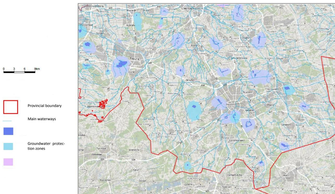
**Figure 3: Ground water protection zones for drinking water intake.**
