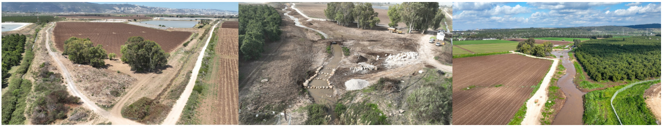
Figure 10: Floodplain reconnection and river channel restoration as a measure that can help reduce flood risk (before/ during/ after implementation. Source: MERLIN Case Study 15 (Tzipori catchment, Israel))
