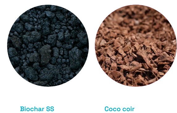
Figure 3.1 Selected substrates in the NICE project with notable adsorption capacities for emerging contaminants.
