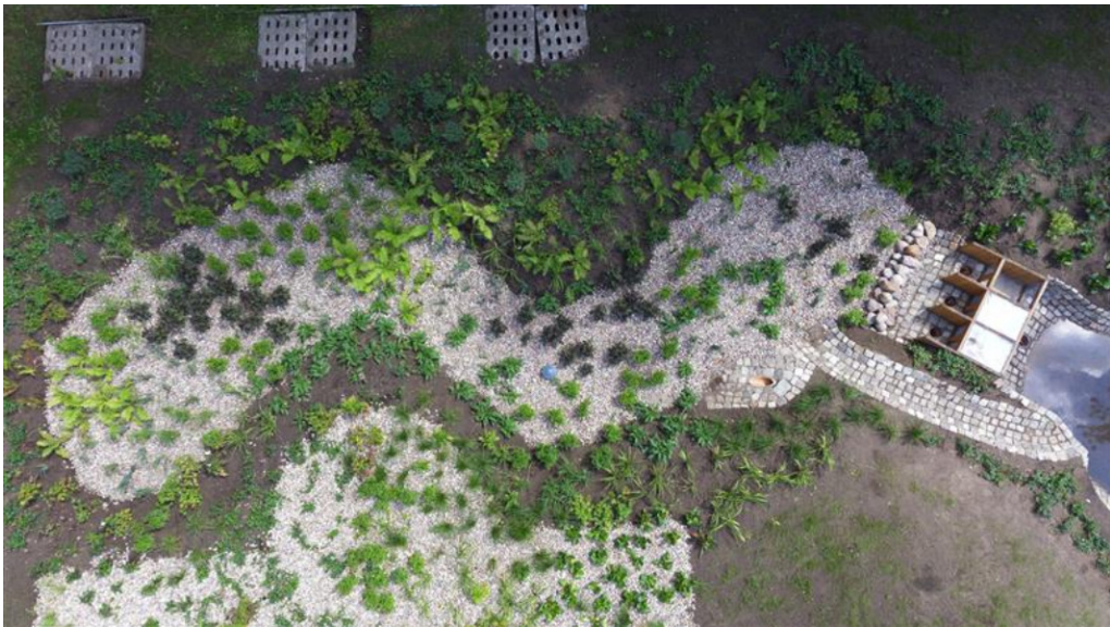
Figure 9 Rain garden after implementation, showing functional and hydrological vegetation zones.
